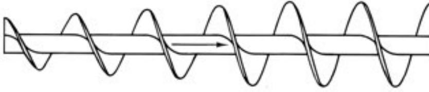
**Tapering flight conveyor screw**
