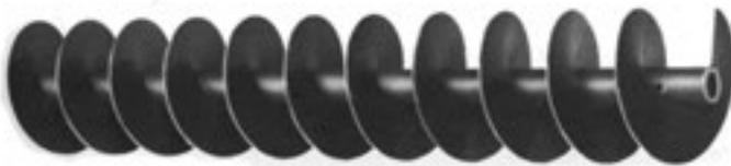
**Short pitch conveyor screws** are of regular construction except that the pitch of the flights is reduced. They are recommended for use in inclined conveyors of 20 degrees slope and over, including vertical conveyors and are extensively use as feeder screws. They retard flushing of materials of a fluid nature.
