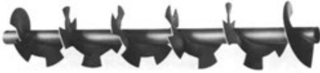
**Cut flight conveyor screws** have notches cut in the periphery of either helicoid or sectional flights. These notches supplement the conveying action with a moderate mixing action. They are used for light, fine, granular or flaky materials.
