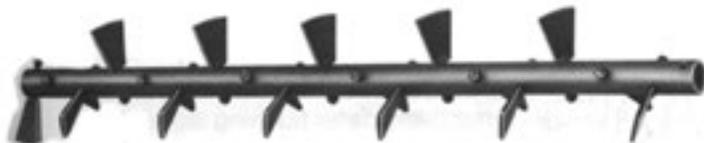
**Paddle conveyor screws** have formed steel blades mounted on rod shanks inserted through the pipe. Conveying action can be controlled by adjusting the angle of the paddles. They are used for mixing, blending or stirring dry or fluid materials.
