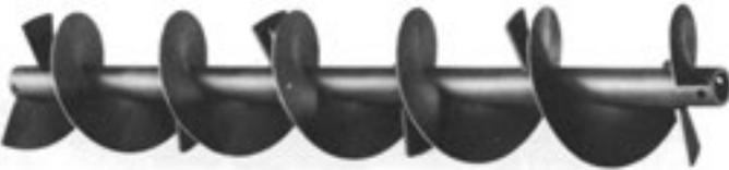
**Conveyor screws with paddles** have paddles spaced at intervals and set to partially oppose the forward flow, to provide a moderate mixing or stirring of materials being conveyed. Paddles are adjustable and may be set at any angle to produce the desired degree of agitation. They are used for light or medium weight, fine, granular or flaky materials.
