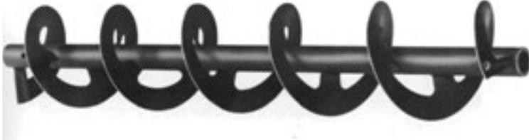
**Ribbon flight conveyor screws** consist of continuous helical flighting formed from steel bar and secured to the pipe by supporting lugs. They are used for conveying sticky, gummy or viscous substances, or where the material tends to stick to flighting at the pipe.
