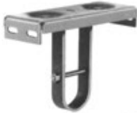
**No. 216 hangers** have formed steel box frames of superior strength and rigidity and are excellent for heavy service. They are mounted within the conveyor trough. Mounting holes are slotted parallel with the conveyor to permit adjustment and alignment. These hangers are normally furnished with hard iron, babbitted, bronze, oil impregnated wood or molded fabric bearings, but can also be furnished with special bearings.
