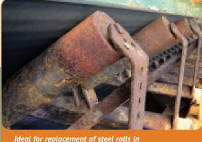
Ideal for replacement of steel rolls in corrosive environments.
