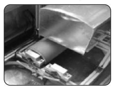
Rolls are weighed. Rolls are partially submerged and rotated. Rolls are weighed again to determine if any water bypassed the seal. This test is per DIN 22112-3.
