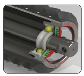
Precision-machined ductile-iron bearing housings provide highly controlled bearing bore dimensions, excellent circular runout and excellent alignment through the roll from end to end. In addition, the high concentricity of the machined bearing housing is transferred to the shell and actually improves the roundness of the shell.
