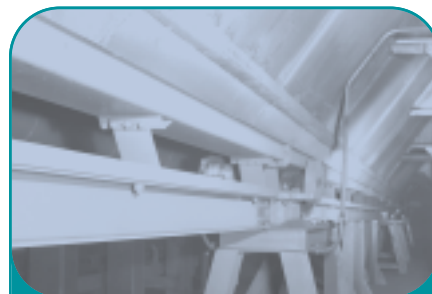
A 12-inch wide by 48-foot long Flexmount conveyor handling 6 TPH of spill sand. Grating and collecting hopper above collects spill sand from molding operation.
