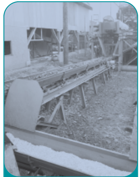
Coilmount vibrating conveyor transferring redwood bark to another Coilmount transfer conveyor.
