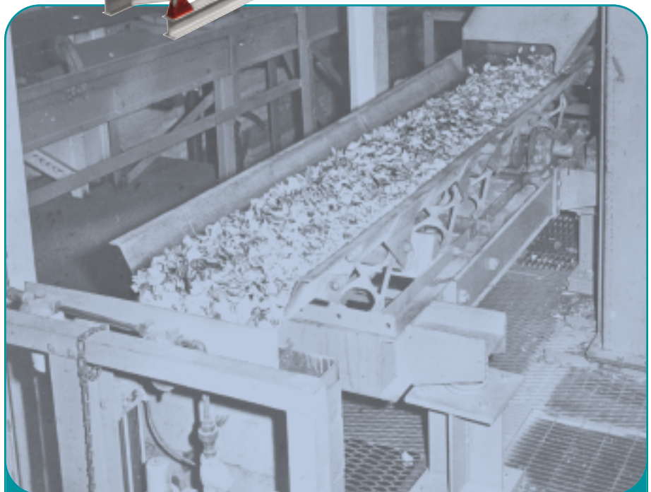
A 20-inch wide Coilmount conveyor handling wood chips. Installed on upper floor of building, the conveyor has a spring mounted and counterweighted base to isolate vibration from building structure.
