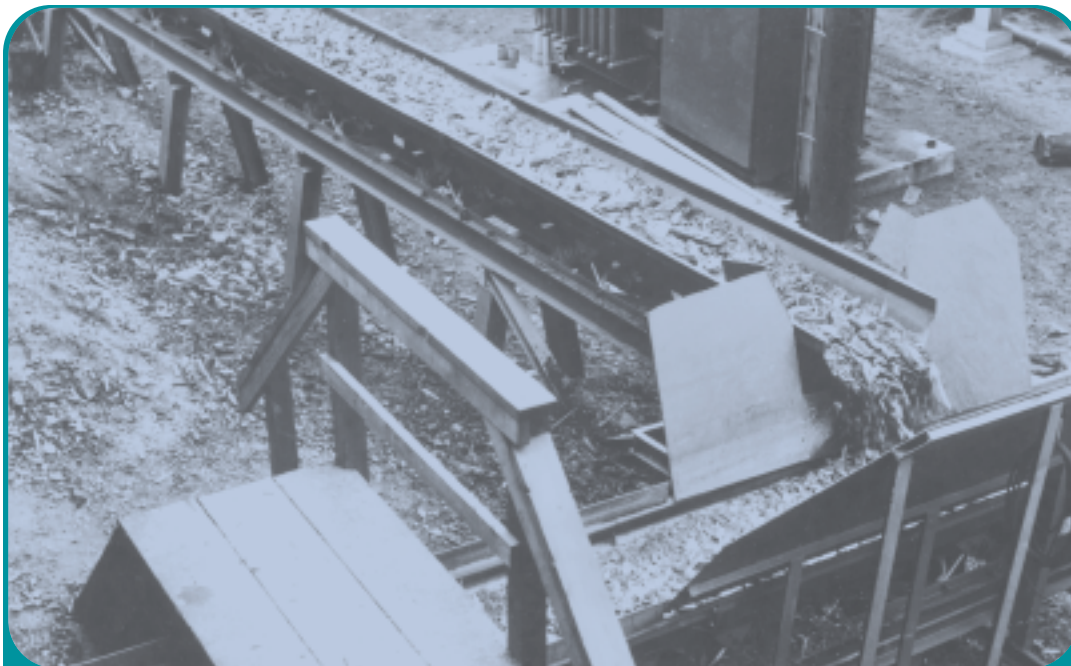
Coilmount conveyor handling redwood bark from a debarker to another Coilmount transfer conveyor.
