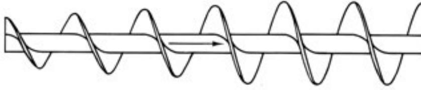
**Tapering flight conveyor screw**
