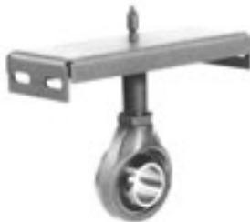
**No. 270 ball bearing hangers** have self-aligning ball bearings. The frame is a box-member top-bar with a pipe stem support for the bearing. The bearing is factory adjusted for the proper length from the top-bar and locked with a sealant and a lock nut. The frame is designed for mounting inside the trough and slotted mounting holes parallel to the conveyor permit adjustment and alignment.
