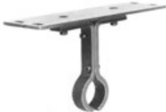
**No. 220 hangers** are similar in construction to No. 226 hangers, except they are mounted on top of the trough flanges. Mounting holes are slotted parallel with the conveyor to provide adjustment and alignment. These hangers are normally furnished with hard iron, babbitted, bronze, oil impregnated wood or molded fabric bearings, but can also be furnished with special bearings.
