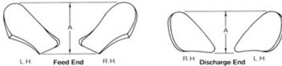
End Lugs are die-formed steel plates welded to both ends of helicoid flighting and to the pipe to strengthen the end of flighting.
