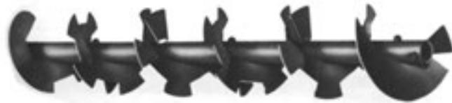
**Cut flight conveyor screws with paddles** have paddles mounted at intervals and set to counteract the flow of materials, considerably increases the agitation and mixing action produced by the cut flights.
