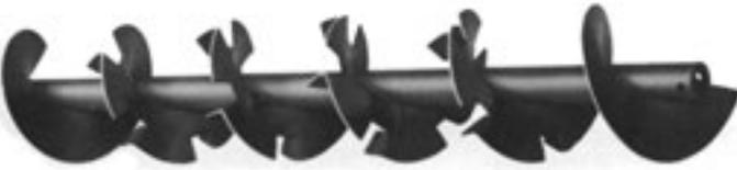
**Cut and folded flight conveyor screws** provide folded segments which act as lifting vanes to produce a cascading effect. This promotes agitation and aeration, resulting in better mixing. They are used for light or medium weight, fine, granular or flaky materials.
