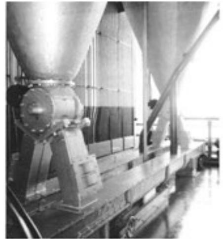
**Bottom:** Helicoid screw conveyors are essential components in this flour collecting system located in a large bakery.
