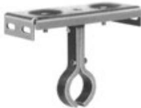
**No. 226 hangers** have a rigid, formed-steel box frame with clearance for passage of material in large volume. They are mounted within the conveyor trough. Mounting holes are slotted parallel with the conveyor to permit adjustment and alignment. These hangers are normally furnished with hard iron, babbitted, bronze, oil impregnated wood or molded fabric bearings, but can also be furnished with special bearings.
