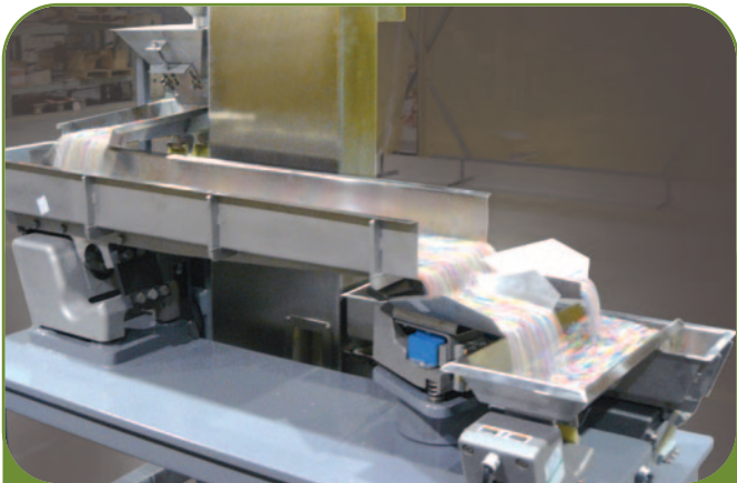
Integrated high stroke system using BF-3, RS drive, BF-2 and a Link-Belt bucket elevator.
