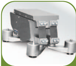
Model BF-4 LF drive will handle up to 110 pound mass with up to .120 stroke.
