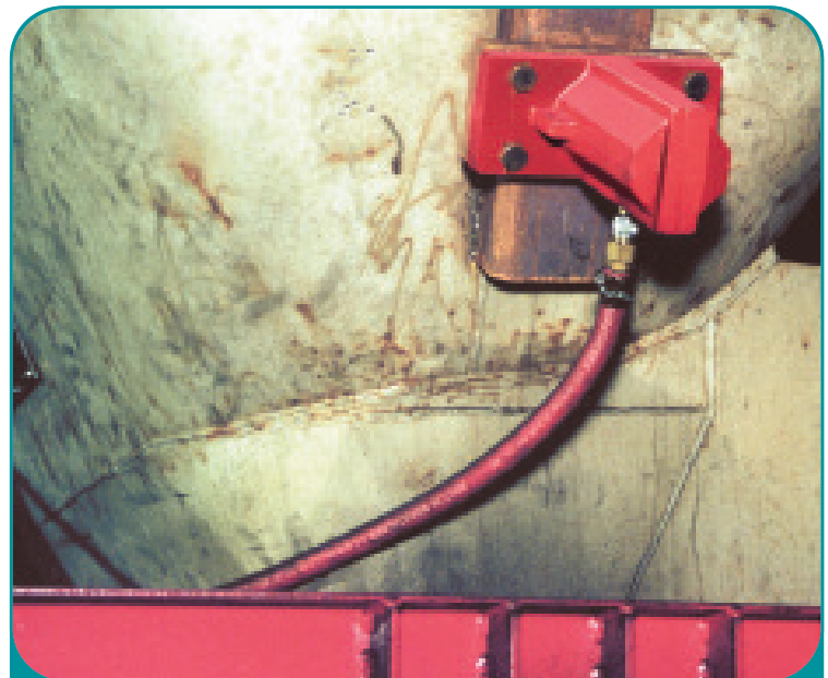
Syntron® Pneumatic Piston vibrator maintains consistent flow of coal from a coal bin to a vibrating feeder.
